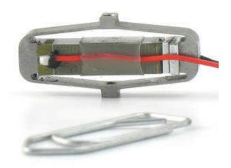
• A linear micro amplifier Caµ10: converts a voltage from [0; 3.3V] to [5; 150V]
